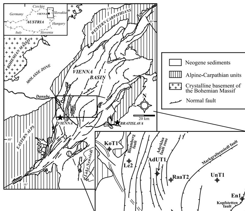
**Fig. 2** Tectonic sketch map of the Vienna Basin (redrawn from Wessely, 1984; Decker, 1996) and locations of studied wells. Abbreviations: KoT1, Korneuburg T1; Le2, Leopoldau 2; AdUT1, Aderklaa UT1; RaaT2, Raasdorf T2; UnT1, Untersiebenbrunn T1; En1, Engelhartstetten 1.
