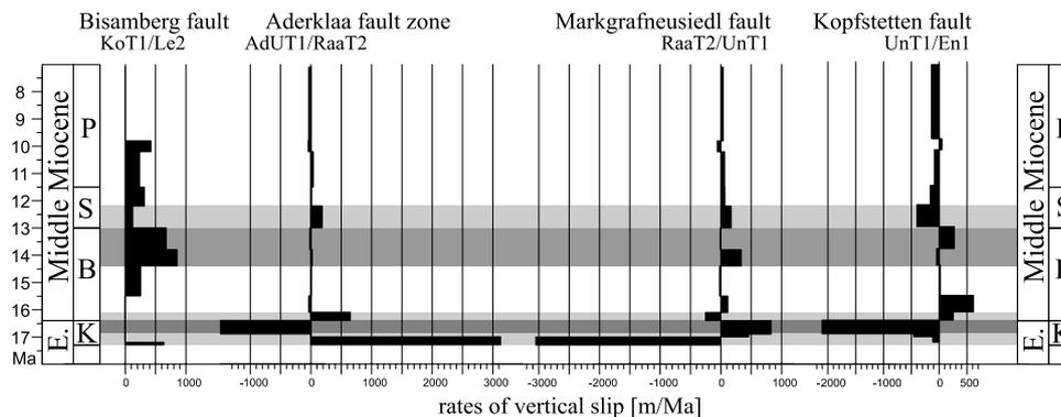
**Fig. 6** Step plot of apparent relative dip-slip rates vs. stratigraphic time for four synsedimentary faults along a Vienna Basin transect from west to east. Interpreted times of main fault activities are marked in grey. E, early Miocene; K, Karpatian; B, Badenian; S, Sarmatian; P, Pannonian.
