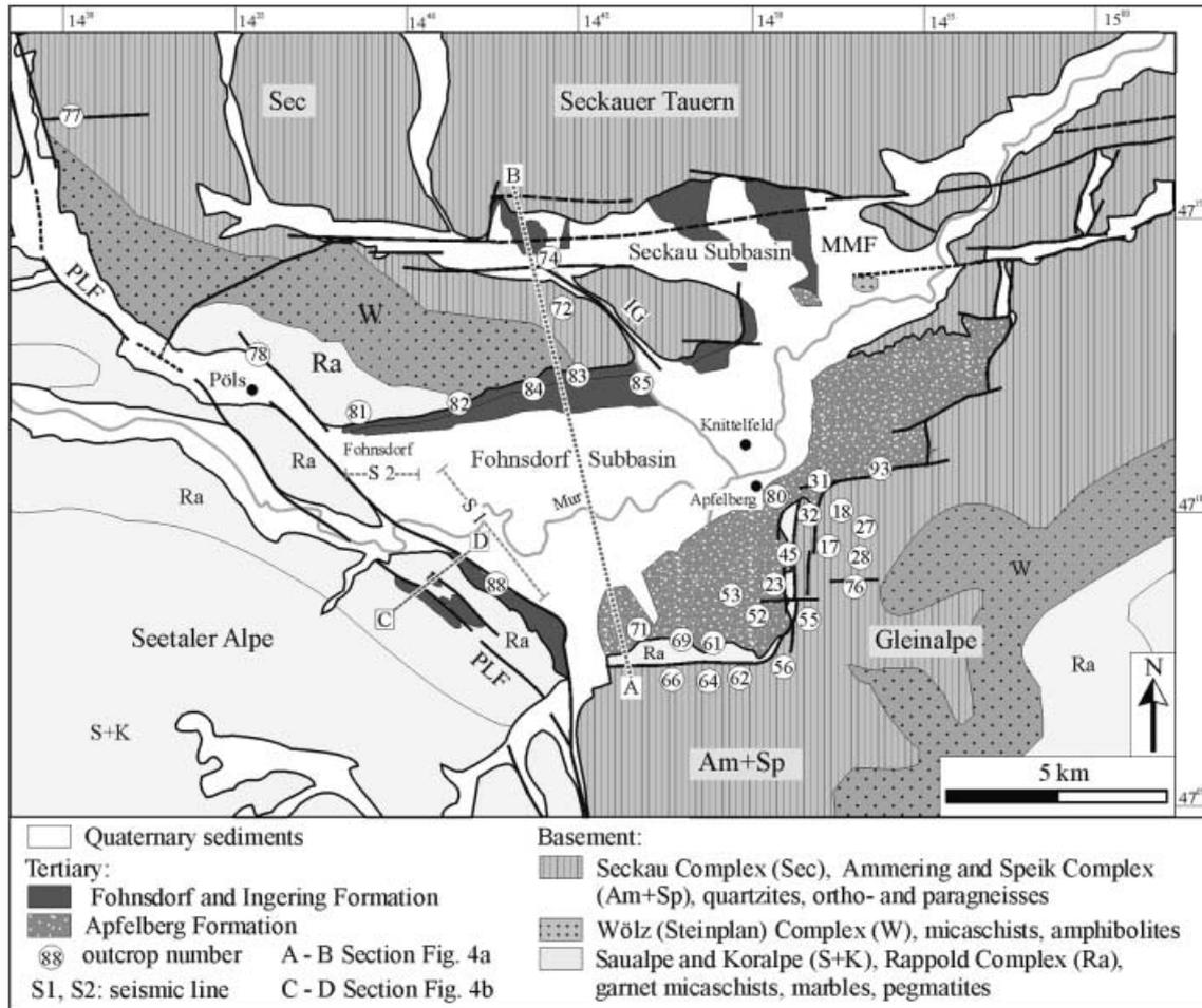
**Fig. 2** Geological map of the Fohnsdorf-Seckau Basin and the surrounding basement. *Numbers* refer to outcrops used for tectonic analysis. Note repetition of Rappold complex (*Ra*) due to normal faulting along the SE basin margin. Synthesized from maps by Polesny (1970), Flügel and Neubauer (1984), Schuster et al. (1999) *PLF* Pöls-Lavanttal fault system, *MMF* Mur-Mürz fault system, *IG* Ingering fault
