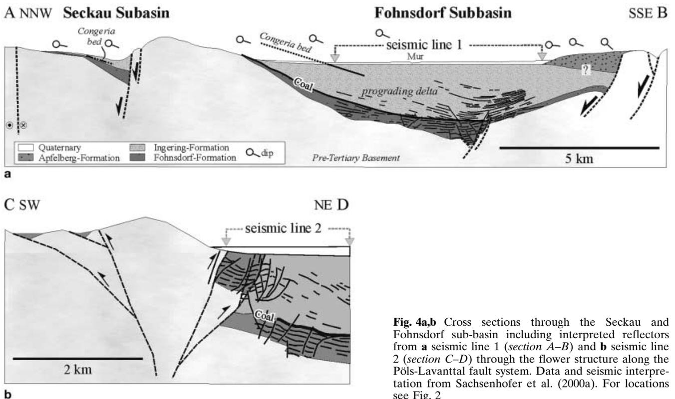
**Fig. 4a,b** Cross sections through the Seckau and Fohnsdorf sub-basin including interpreted reflectors from **a** seismic line 1 (section A–B) and **b** seismic line 2 (section C–D) through the flower structure along the Pöls-Lavanttal fault system. Data and seismic interpretation from Sachsenhofer et al. (2000a). For locations see Fig. 2
